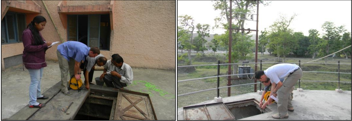
Plate 3.Groundwater level measurement in RBF wells
